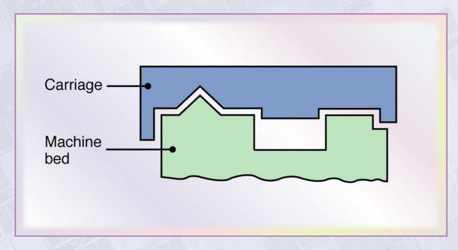
Figure 35.1 Cross-section of a machine-tool slideway. The width, depth. Angles, and other dimensions all must be produced amd measured accurately for the machine tool to function as expected.
