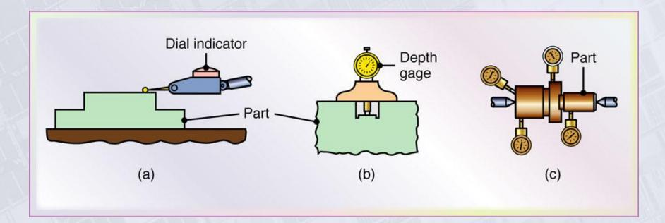
Figure 35.4 Three uses of dial indicators: (a) roundess, (b) depth, and (c) multiple-dimension gaging of a part.
