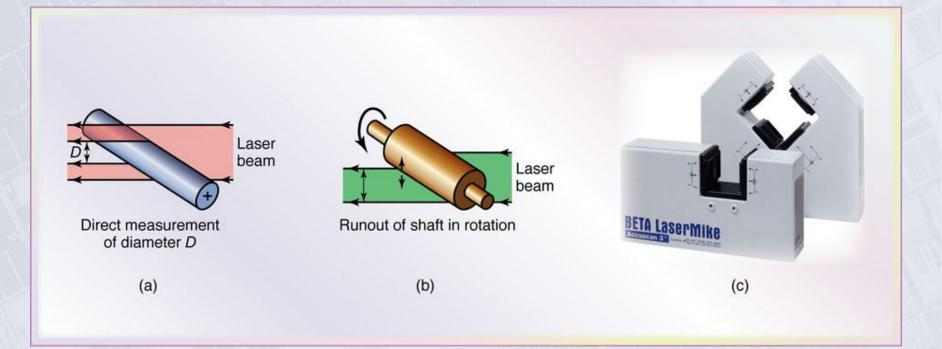
Figure 35.14 (a) and (b) Two types of measurements made with a laser scan micrometer. (c) Two types of laser micrometers. Note that the instrument in the front scans the part (placed in the opening) in one dimension; the larger instrument scans the part in two dimensions. *Source*: Courtesy of BETA LaserMike.
