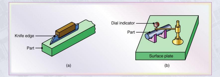
Figure 35.5 Measuring straightness manually with (a) a knife-edge rule and (b) a dial indicator. *Source*: After F. T. Farago.
