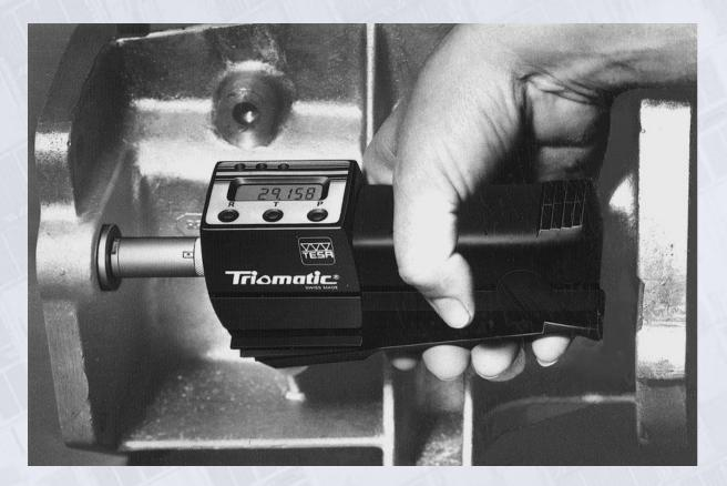
Figure 35.12 An electronic gage for measuring bore diameter. The measuring head is equipped with three carbide-tipped steel pins for wear resistance. The LED display reads 29.158 mm. *Source*: Courtesy of TESA SA.
