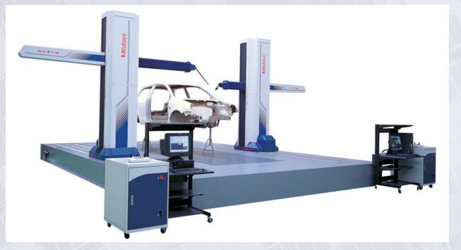
Figure 35.16 A large coordinate-measuring machine with two heads measuring various dimensions on a car body. *Source*: Courtesy of Mitutoyo Corp.
