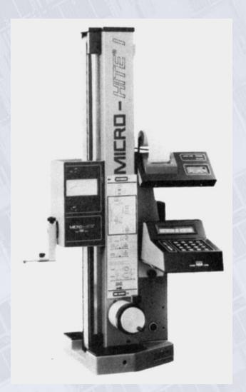
Figure 35.13 An electronic verticallength measuring instrument with a resolution of 1  $\mu$ m (40  $\mu$ in). *Source*: Courtesy of TESA SA.
