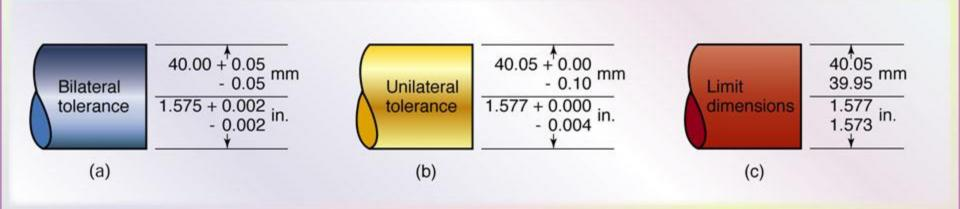
Figure 35.18 Various methods of assigning tolerances on a shaft: (a) bilateral tolerance, (b) unilateral tolerance, and (c) limit dimensions.
