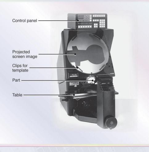
Figure 35.9 A bench-model horizontal-beam contour projector with a 16-in. diameter screen with 150-W tungsten halogen illumination. *Source*: Courtesy of L. S. Starrett Company, Precision Optical Division.
