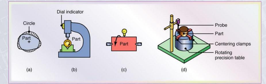
Figure 35.7 (a) Schematic illustration of out-of-roundess (exaggerated). Measuring roundess using (b) a V-block and dial indicator, (c) a round part supported on centers and rotated, and (d) circular tracing. *Source*: After F. T. Farago.
